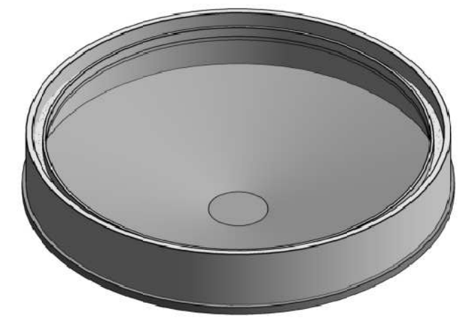
IMAGE OF SLUDGE THICKENER
